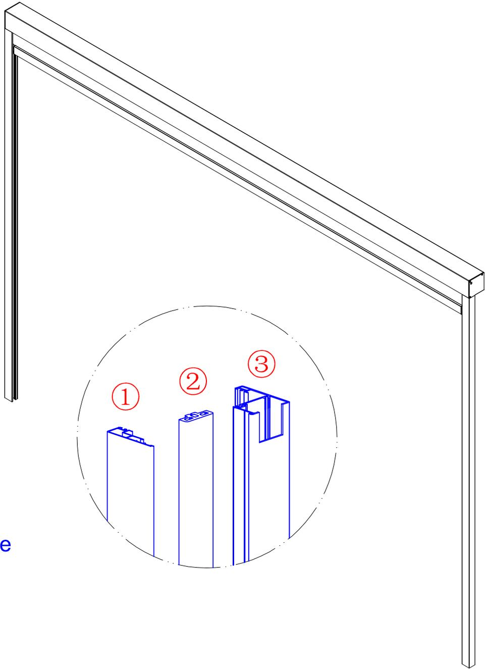
7. Take apart the pre-assembled side rails into 3 pieces ①-②-③ and you can slide out the part No.① easily by hand.
