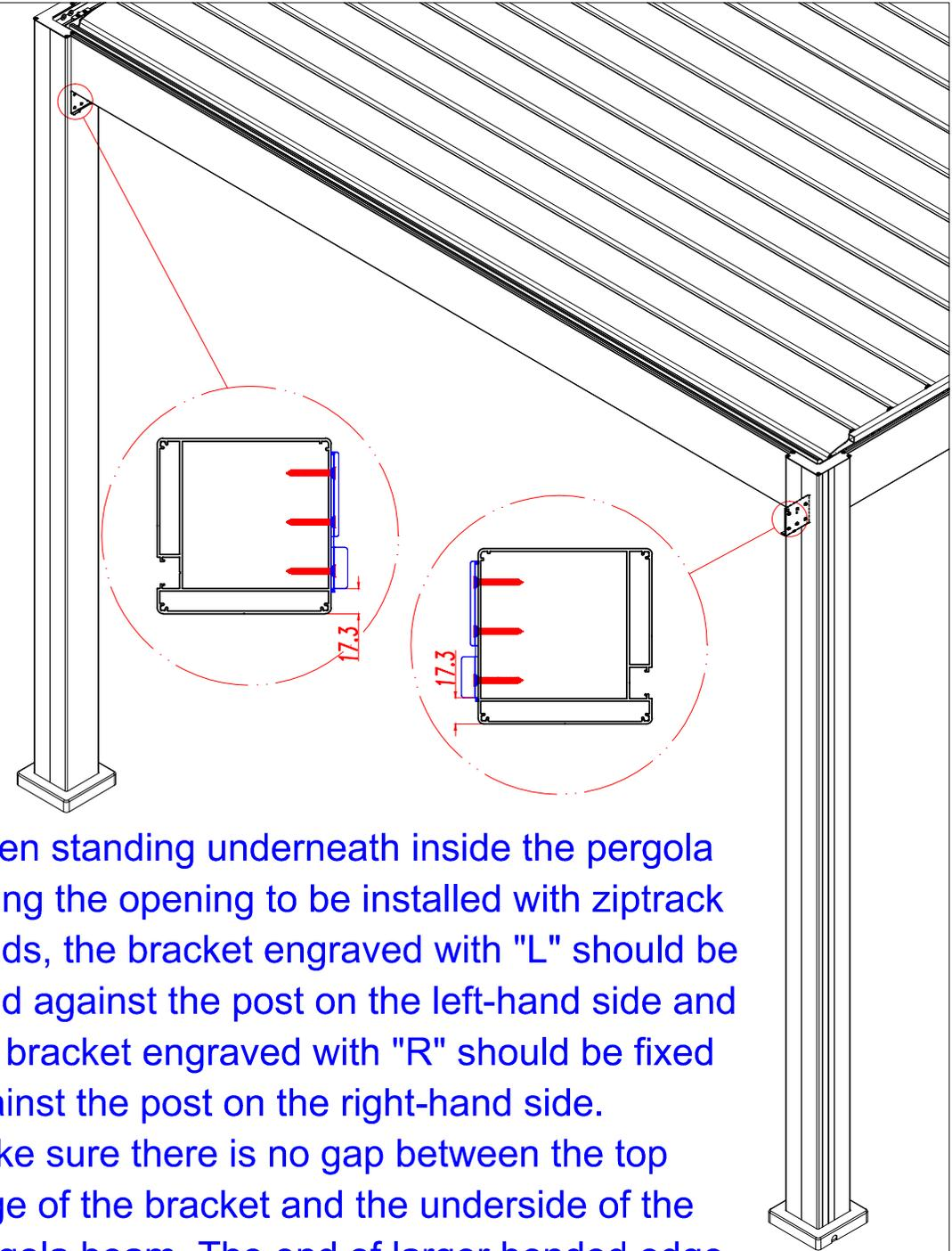
3. When standing underneath inside the pergola facing the opening to be installed with ziptrack blinds, the bracket engraved with "L" should be fixed against the post on the left-hand side and the bracket engraved with "R" should be fixed against the post on the right-hand side.
