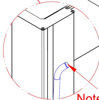
Note: the pvc pipe here should be fitted into the wire inlet hole without any protruding out. Then fix it in place with glue.
