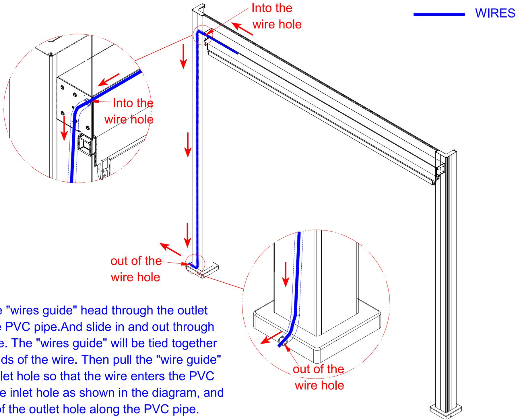
6. First, put the "wires guide" head through the outlet hole into the PVC pipe. And slide in and out through the inlet hole. The "wires guide" will be tied together with both ends of the wire. Then pull the "wire guide" from the outlet hole so that the wire enters the PVC pipe from the inlet hole as shown in the diagram, and comes out of the outlet hole along the PVC pipe.
