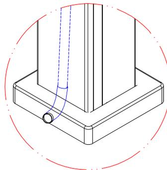
The hole of the base plate cover should be cut on site
