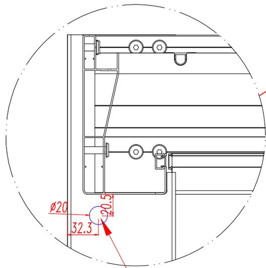
Here the inlet hole of the post needs to be cut on site
