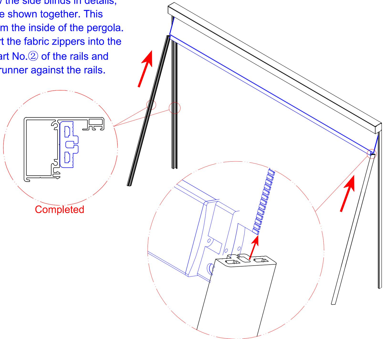
12. Clip in the part No.① into part No.③ by using the rubber mallet. Knock firmly from the top first and then all the way down to the ground. Installation will be completed when there's no gap between the part No. ① and the part No.③.
