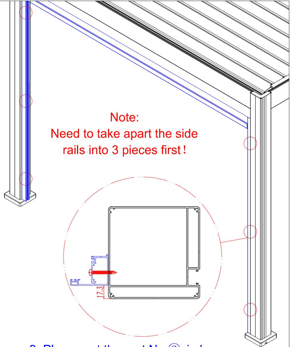
9. Please set the part No.③ in by 17.3mm from outside the post and then fix the side track with 3 screws from top, middle and bottom position.
