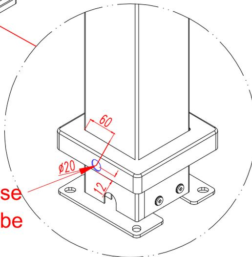
1. As shown, the post and base plate cover should be cut with a slot hole in diameter 20mm.
